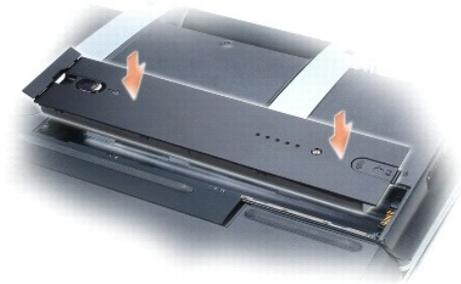
3. Slide the battery in the direction of the #1 arrow until it snaps into place.
