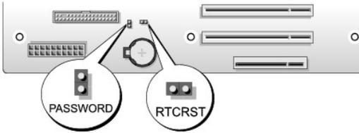
3. Locate the 2-pin password jumper (PASSWORD) on the system board (see [System Board Components](#)), then remove the jumper plug and set the plug aside.
