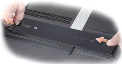
c. Lift the battery straight up and out of the computer.
